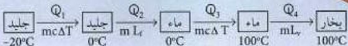
$$Q_1 = m c_1 \Delta T_1 = 50 \times 10^{-3} \times 2100 \times (0+20) = 2100 \text{ J}$$
