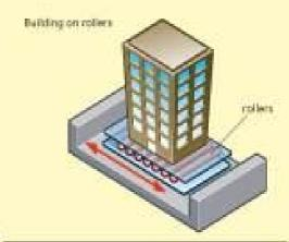
It is probably impossible to design a building that would be completely secure in the most senious earthquake. It would also be very costly. Instead, engineers design buildings which will not fall down when the earth quakes. There are two main ways of doing this. First, buildings are built on springs or rollers, so that when the earth quakes, the building itself moves a little. Another method is to use building materials that soften the impact of an earthquake.
